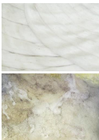
Fig. 2: The sliver feed (top) and the dirt particles (bottom) eliminated during spinning show that the good fibers are fully utilized. The optimized air flow and the improved fiber guidance in the S 36 spin box form the basis for this.
