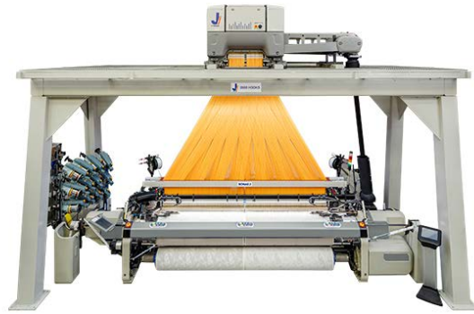
Figure 1: Ji2 jacquard with 2.688 hooks on a rapier loom weaving designs on double width in 8 repeats
