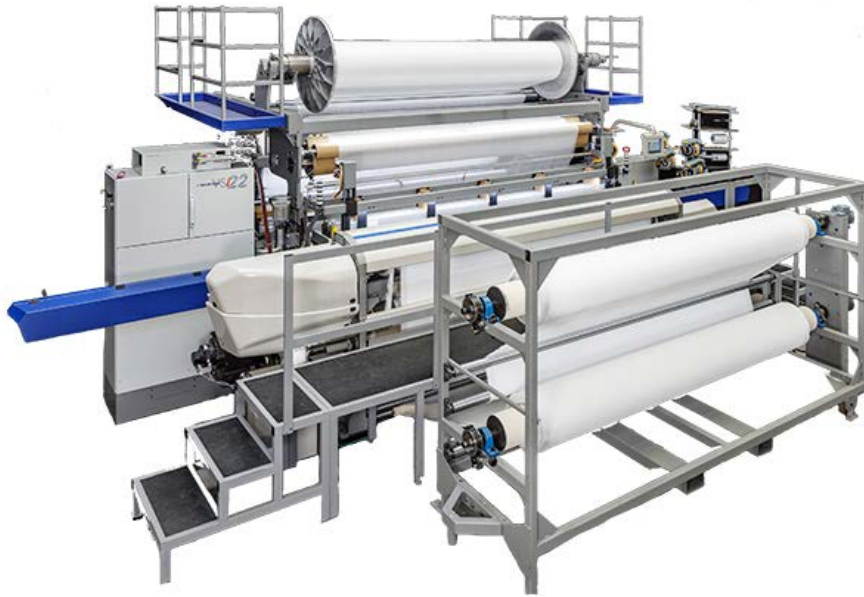
Figure 3: VSi22 Velvet Smart Innovator for weaving plain velvet on 3 meters width
