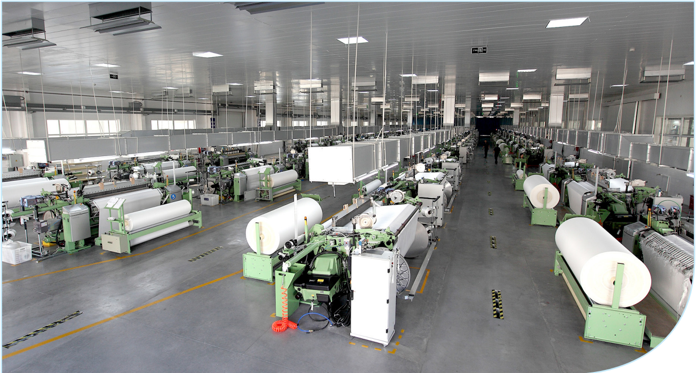
Quality and precision: This is where precision filter fabrics for liquid, solid and air filtration are produced on rapier weaving machines from the house of DORNIER (Photo: "Weaving mill"; Source: DORNIER)
