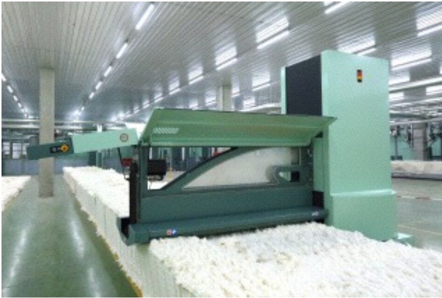
Six UNifloc A 12 bale openers supply the compact spinning machine K 46
