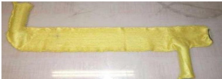
3D knitted preform at final dimension
