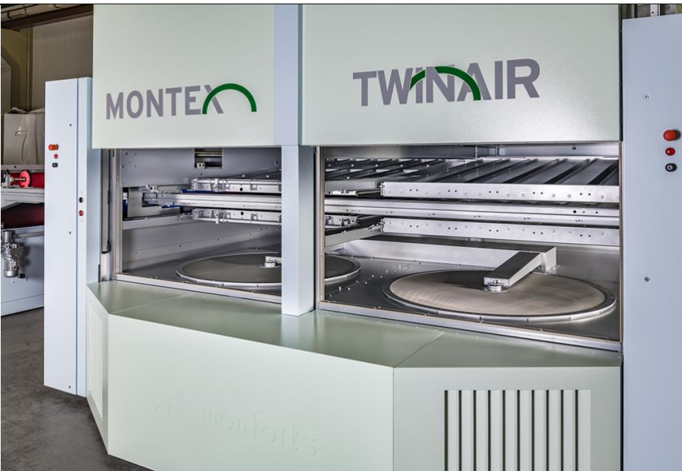
On the Monforts TwinAir system, the airflows above and below the fabric being dried can be regulated completely independently of each other.
