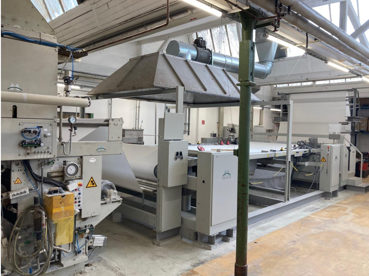
Two almost identical Monforts sanforizing lines now provide Wülfing with much improved flexibility.
