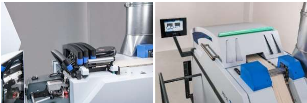
The DISC MONITOR system measures the count continuously. The T-LED display provides visual indications of the machine's status over a large distance.
