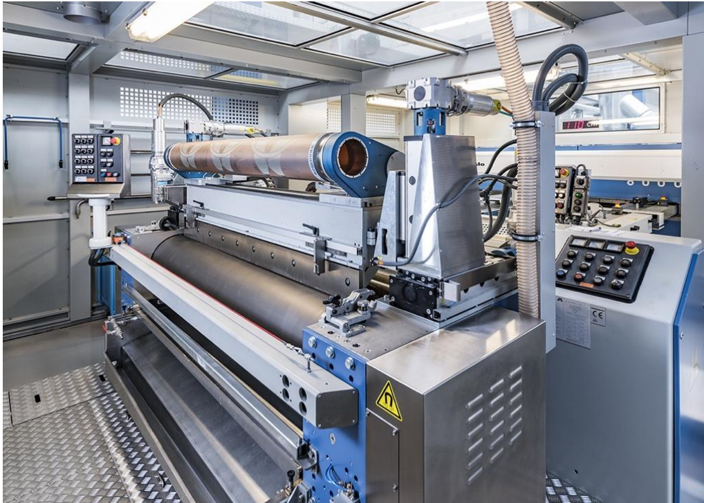
Montex®Coat unit integrated into the full technical textiles pilot line at the Monforts ATC.
