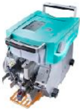
TIEPRO warp tying installation
