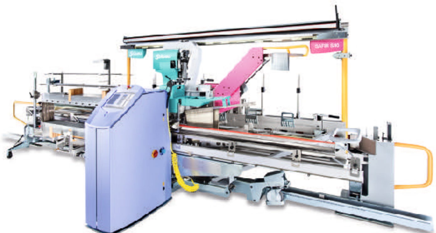
SAFIR S40 automatic drawing-in machine
