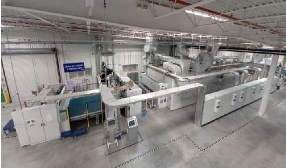
Photo 1: SUPRA FLOW BX double-belt thermofusion oven with rotary longitudinal cutter, guillotine cross cutter and semi-automatic winder for the production of voluminous nonwovens for the furniture industry
