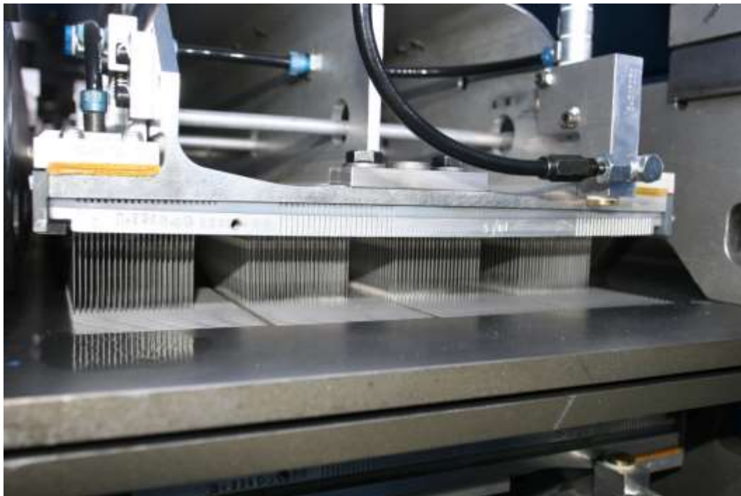
Photograph shows the container board in the MicroPunch needleloom
