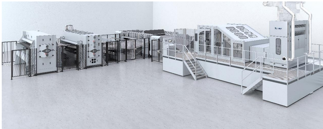
A first T-SUPREMA needle-punching line.
