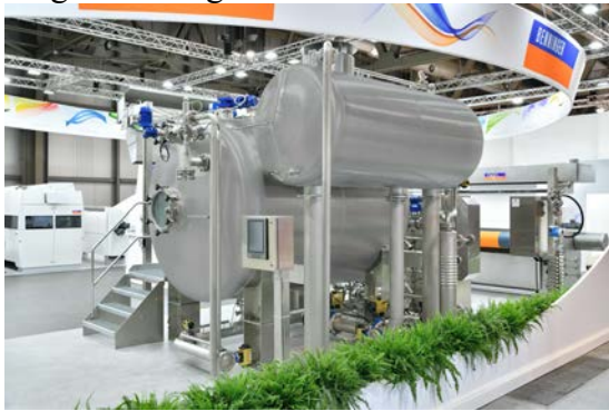
FabricMaster – fast, versatile, and economic jet dyeing machine
