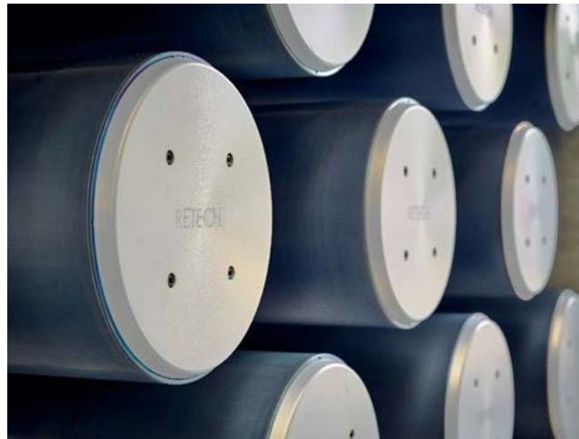
High end heated godet rolls, suited for up to 350°C and ultra-high draw forces
